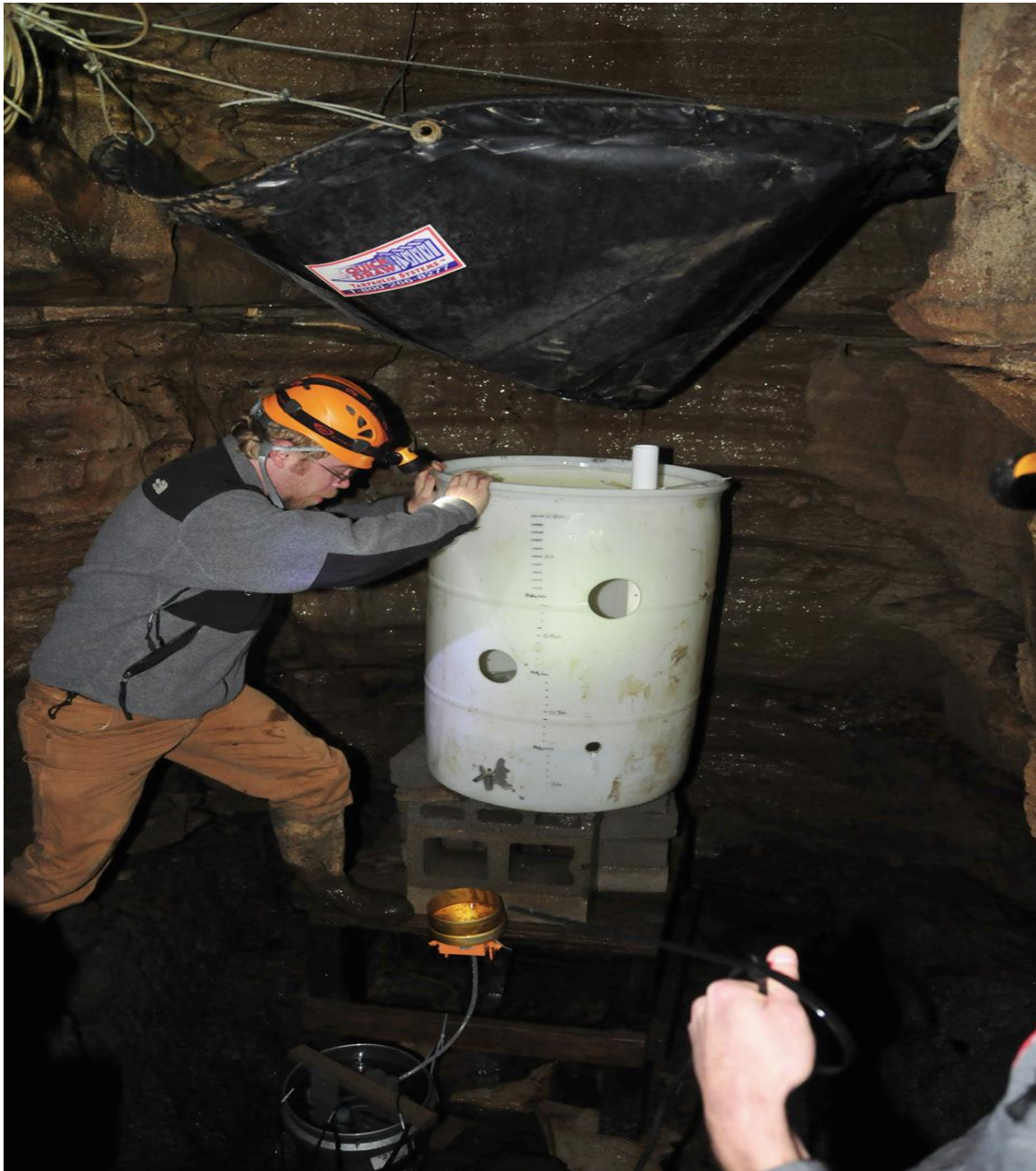
Figure 10. Photograph of barrel-shaped weir at Waterfall 1 in Crumps Cave used for discharge measurements. The water level is measured with a pressure transducer in the barrel and the temperature, pH, and specific conductance probes are in the bucket below (photo by Jason Polk).
